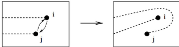
FIG. 3. Elementary braid interchange of two vortices.
