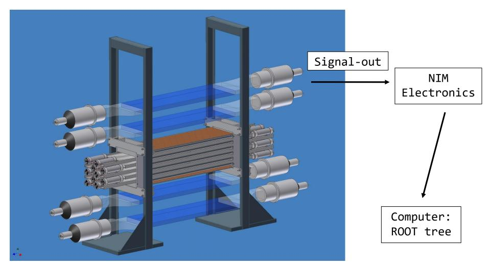
$\rightarrow$  16 PMT signals, w/both energy and timing information, are recorded by the data acquisition system (DAQ). An analyzer program converts the binary data into a ROOT tree.
