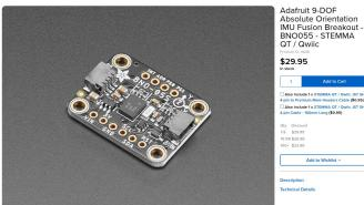
Adafruit 9-DOF Absolute Orientation IMU Fusion Breakout -BNO055 - STEMMA
