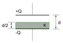
20) If we fix the charge on the capacitor to be  $Q = 6 \times 10^{-11}$  C, what is the potential difference between the top and bottom plates? Note that in the region containing the dielectric medium, the electric field is  $E = E_0 / \kappa$ , where  $E_0$  is the electric field in vacuum.
