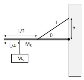
A horizontal rod of length L and mass  $M_R = 2.3$  kg is used to hang a sign on a wall. The right end of the rod is attached to the wall by a hinge. A wire having tension T runs from the center of the rod to a place on the wall a distance h above the hinge as shown. The wire makes an angle  $\theta = 24^{\circ}$  with the rod. The sign has mass  $M_S = 0.767$  kg and hangs distance L/4 from the end of the rod. The system is in equilibrium.
