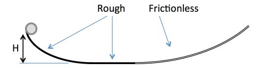
23) If the spherical shell now enters a **frictionless** ramp on the other side as shown, how does the new height it reaches, h, relate to the original height, H, from which it was released?
