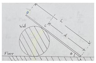
17) Calculate the magnitude of the force  $F_c$  from the cylindrical wall <u>on</u> the beam (at point C).
