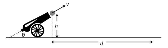
A cannon inclined at an angle of  $\theta = 28^{\circ}$  from the horizontal fires a projectile into the air, as shown in the figure. The projectile exits the cannon at a height h = 1.3 m from the ground and at a speed v = 7 m/s.
