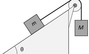
11) What must the mass M be for the blocks to remain at rest?
