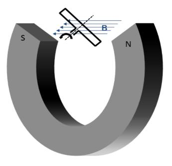
A coil of wire turns between the poles of a permanent magnet as shown in the diagram. The coil has N=34 turns of wire. The magnet produces a constant field of magnitude B = 0.119 T. The coil has a cross-sectional area A = 0.0411 m<sup>2</sup>.
