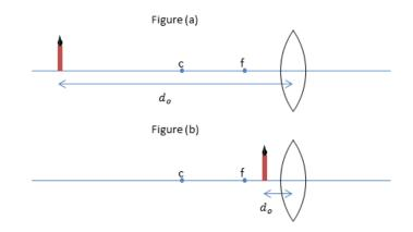
6) The candle is first placed at a distance  $d_o = 14.8 \text{ cm}$  as shown. The image is located at
