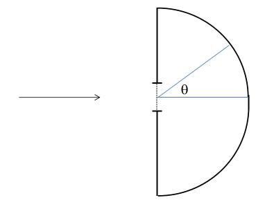
24. A diffraction grating spectrometer has a diffraction grating and a cylindrical screen. The diffraction grating has 8257 slits/cm. Light impinges on the diffraction grating. At which angle  $\theta$  is the 3<sup>rd</sup> order maximum for violet light ( $\lambda = 390$  nm)?
