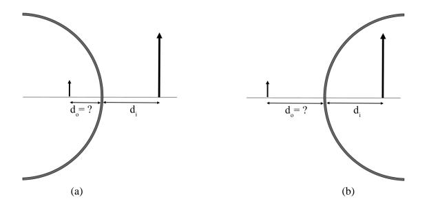
2. A virtual image is formed 15 cm behind a mirror. The image's magnification m is measured to be +5. Determine whether the mirror is concave or convex.
