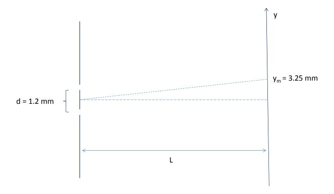
21. A double slit experiment has two slits separated by a distance d = 1.2 mm. Monochromatic (single-wavelength) light is impinging on the two slits with an unknown wavelength. A screen a distance L = 2.5 m away has a third interference maximum (m = 3) at y = 3.25 mm. What is the light's wavelength?
