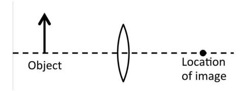
18. Where must one put an object with respect to the convex lens (which has focal length f), so that the image is at the same distance from the lens as the object?
