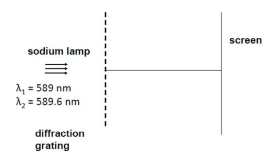
14. At what angle is the first-order maximum for the emission line with a wavelength of 589.0 nm observed?
