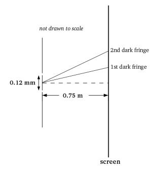
25. What is the distance,  $y_2 - y_1$ , between the first and second dark fringes located from the central axis? Assume the distance between the fringes on the screen is much smaller than the slit-to-screen distance (that is,  $y_2 - y_1 \ll 0.75$  m).
