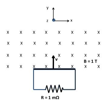
13. From Lenz's rule, what is the relation between the currents induced in the metal frame on entrance to and upon exit from the magnetic field?
