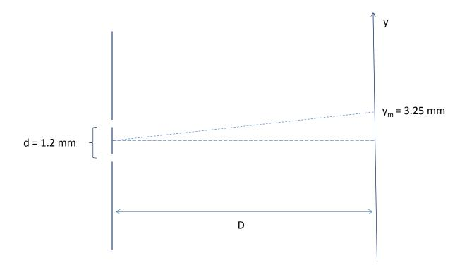
22. The screen is now moved to a new distance D. A different light source of wavelength 50 nm impinges on the two slits. A maximum of order m = 2 now occurs at y = 3.25 mm. What is the new distance D of the screen from the double slits?
