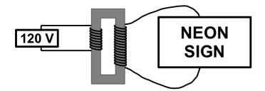
The transformer is designed to have an output voltage of 1200 V when the primary is connected to a 120 V source. How many turns must the secondary winding have if the number of primary turns is 50?
