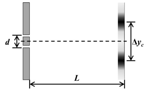
18) What is the distance L if the width of the central bright spot of the interference pattern is  $\Delta y_c = 1.9$  cm.
