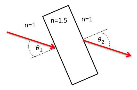
If the angle  $\theta_1$ =60 degrees, what is  $\theta_2$ , the angle with respect to the normal on the side of the glass where the beam exits?
