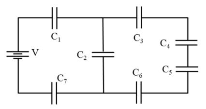
Seven identical capacitors with capacitance C = 8.5 nF are connected to a 12 Volt battery as shown in the figure above.
