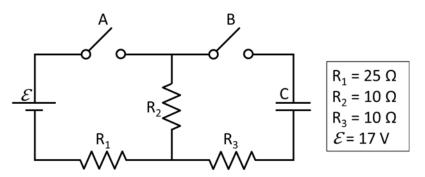
If it takes 12  $\mu$ s for the charge on the capacitor to drop the 1/2 of its initial value, what is the capacitance of the capacitor C?
