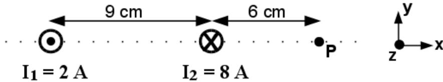
18. Calculate the net magnetic field in the y direction at the point P.
