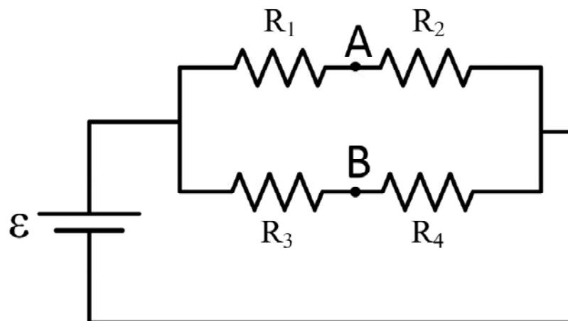
8. If all four resistors have resistance  $R$ , what is the total equivalent resistance for this circuit?
