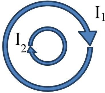
3. Suppose a smaller diameter solenoid is placed inside a larger diameter solenoid, as shown in the top-down view above. The first has current  $I_1$  and turns per unit length  $n_1$ . The second has current  $I_2$  and turns per unit length  $n_2$ . Both currents are in the clockwise direction. What is the magnitude of the magnetic field at the center of the solenoids?
