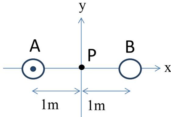
5. If the current through wire A is 1 A and no current flows through wire B, what is the magnitude of the magnetic field at point P?
