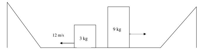
A block sits at rest on a horizontal surface. It suddenly explodes and breaks into two pieces as shown. A piece of mass 3 kg goes to the left and a piece of mass 9 kg goes to the right. Each block slides along the <u>frictionless</u> surface, then up a <u>frictionless</u> ramp. The speed of the 3 kg block is 12 m/s immediately after the explosion.
