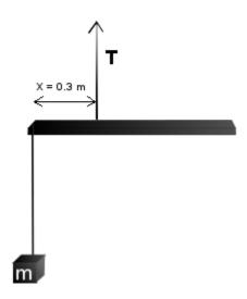
A uniform, one meter board with a mass of 13 kg hangs by a rope X = 0.3 m from the left end of the board with tension T. A box of mass m hangs from the left end of the board.
