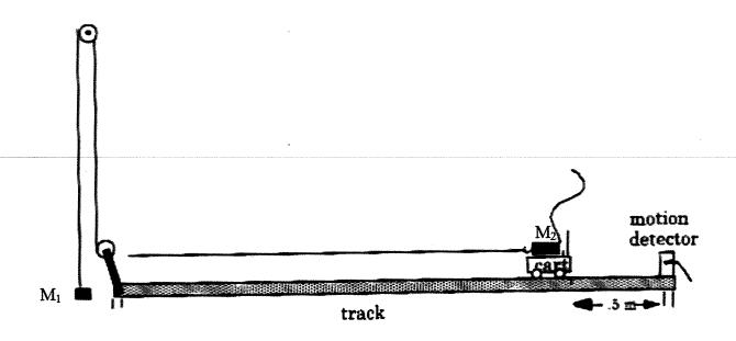
23. In the diagram above, a mass  $M_1$  is pulling a cart of mass  $M_2$ , on a system that has <u>no</u> friction. Depending on whether  $M_1$  is larger or smaller than  $M_2$ , the acceleration of  $M_2$  can be larger or smaller than g.
