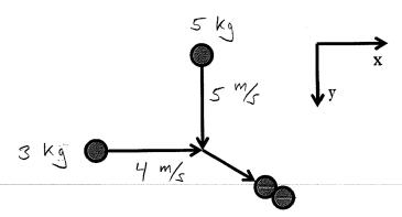
8. There is no gravity in this problem; it takes place on a spaceship in deep space. Two clay balls are thrown. Ball #1 has mass 3.0 kg and velocity 4 m/s in what is called the x direction. Ball #2 has a mass 5.0 kg and is thrown at 5.0 m/s in what is called the y direction (perpendicular to the x direction). They hit and stick. What is the x component of the velocity of the combined mass of clay after the collision?
