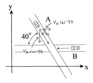
19. What is the velocity vector of car A in components with respect to the designated coordinate system?
