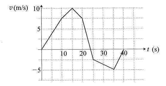
$$a = \frac{V_F - V_i}{t} = \frac{-2.5 - 7.5 \, \text{M/s}}{5} = -2 \, \text{M/s}^2$$
