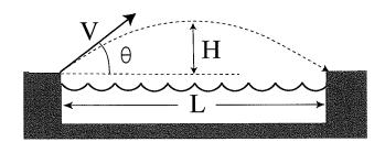
17. The height of the highest point from the ground (above the mid point of the moat) is H = L/3. What is the angle  $\theta$ ? [Hint: Pay attention to the time t required for the ball to reach the highest point. Notice that  $2H = gt^2$  and  $V \sin \theta = gt$ .]
