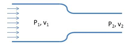
An incompressible and non-viscous ßfluid flows from left to right through a circular pipe that changes its radius from  $r_1$  to  $r_2$  between regions 1 and 2 (see figure above, not to scale). The fluidic velocity in region 1 is  $v_1$  (=3 m/s) and the fluidic velocity in region 2 is  $v_2$  (=9 m/s). The density of fluid is 1,300 kg/m<sup>3</sup>.
