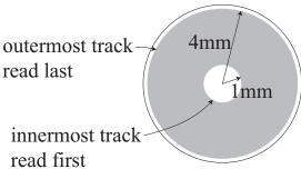
18. For the outermost track, what is the linear reading speed? (The linear reading speed is the constant tangential speed which is maintained while playing the disk.)
