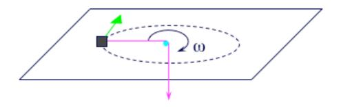
22. A puck of mass 0.2 kg slides in a circular path on a horizontal frictionless table at an angular speed  $\Box$  of 10 rad/s. It is held at a constant radius of 1 meter by a string threaded through a frictionless hole at the center of the table. Then, you pull on the string such that the radius decreases by a factor of 3. What happens to the angular speed of rotation?
