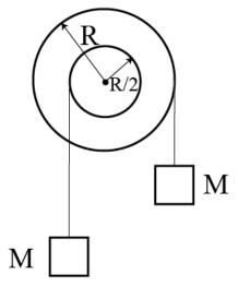
4. The masses start to move and the pulley starts to rotate from the initial stationary condition. M = 1.2 kg and R = 1.5 m. When the right mass goes down by 1m, what is the total kinetic energy of the system? Notice that the distance the left mass moves is just half of the right mass.
