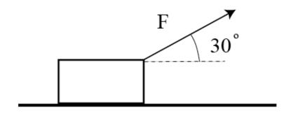
19. A box sits on the floor. A force F = 200 N is then applied to the right but slightly upward at an angle of 30 deg from the horizontal (see diagram) such that the box moves 5 meters horizontally to the right. How much work is done by the force?
