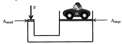
12. The two pistons are initially at the same height. What force F must be applied to the small piston to support the car?
