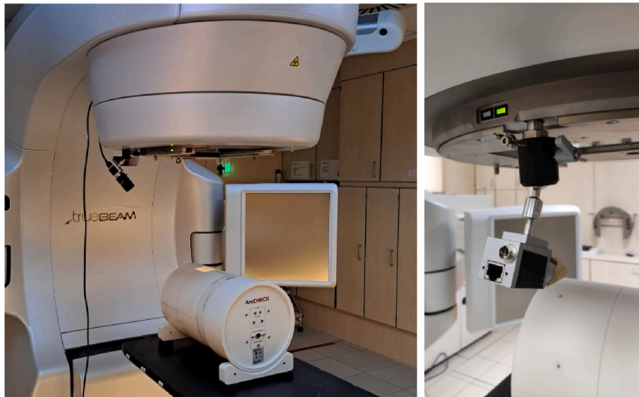
Fig. 2. Camera placed at the head of the LINAC, facing the beam's isocentre.
