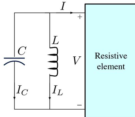
The voltage  $V$  across the resistive element and the current  $I$  flowing into it are related via a nonlinear voltage-current characteristic  $I = g(V)$ .
