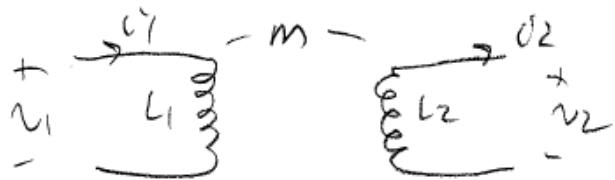
$$120\sqrt{2} \cos 2\pi 60t = L_1 \frac{di_1}{dt} \pm m \frac{di_2}{dt} \quad \text{open circuit}$$
