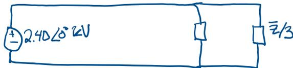
$$S_{1,\phi} = 100 \text{ kVA}, \text{ PF} = 1$$
