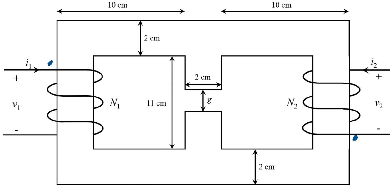
Two coils are wrapped around an iron core with the given dimensions and depth of 3 cm into the page. Coil 1 contains 400 turns and Coil 2 contains 200 turns. The iron has a permeability  $\mu=1500\mu_0$  and contains an air gap of  $g=4$  mm. Fringing effects can be neglected.
