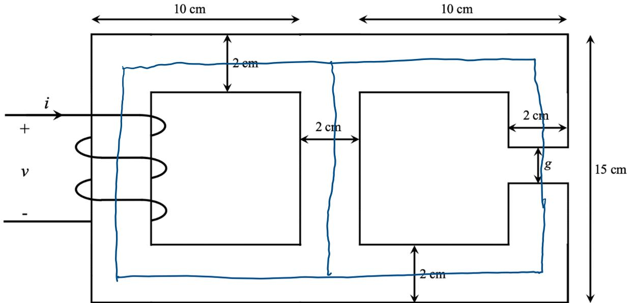
A coil is wrapped 300 times around an iron core with the given dimensions and a depth of 2 cm into the page. The iron has a permeability  $\mu=2000\mu_0$  and contains an air gap of  $g=2$  mm. Fringing effects can be neglected.
