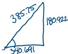
$$\begin{aligned} \theta_n &= \cos^{-1}(0.975) \\ \theta_n &= 12.84^\circ \\ Q_n &= P \tan(\theta_n) \\ Q_n &= 77.65 \text{ kVAR} \end{aligned}$$
