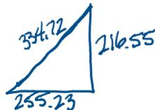
$$\begin{aligned} \theta_n &= \cos^{-1}(0.99) \\ \theta_n &= 8.11^\circ \\ Q_n &= 255.23 \tan(8.11^\circ) \\ &= 36.37 \text{ kVAR} \\ \bar{S}_n &= 255.23 + j36.37 \text{ kVA} \\ &= 257.81 \angle 8.11^\circ = \sqrt{3} V_L I_L \angle \theta \\ \bar{I}_L &= 310.1 \angle -8.11^\circ \end{aligned}$$
