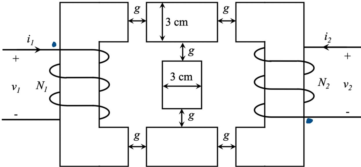
Two coils are wrapped around an iron core with infinite permeability as shown. Coil 1 has 200 turns while coil 2 has 100 turns. The air gap  $g$  is 10 mm and the depth into the page is 3 cm. Neglect fringing.
