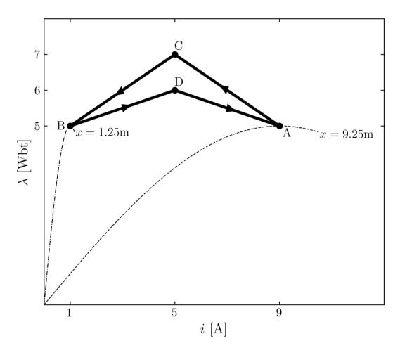
c) If the system moves from point B back to point A through point D (i=9 A,  $\lambda=6$  Wbt) along the lines shown, what is the EFE over this cycle? Does the system behave like a motor or a generator over this cycle?
