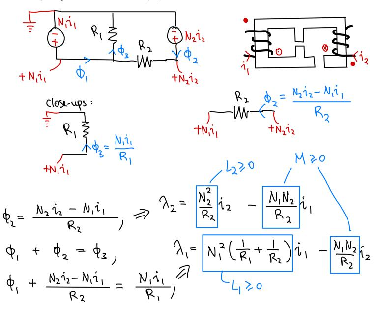
$$L_{1} = \frac{N_{1}^{2}(R_{1}^{-1} + R_{2}^{-1})}{1 + R_{2}^{-1}} = 2.1 H$$
