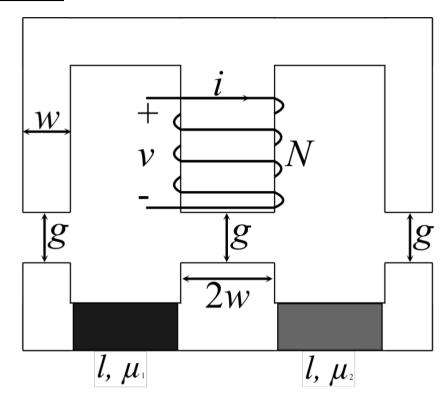
An iron core with infinite permeability, width w=2 cm, air gap length g=3 mm, and depth into the page d=3 cm has a coil wrapped around it as given above with N=250. The iron core also has two inserts in it with length l=10 cm and permeabilities  $\mu_1=2500\mu_0$  and  $\mu_2=1250\mu_0$ . Fringing effects can be neglected.
