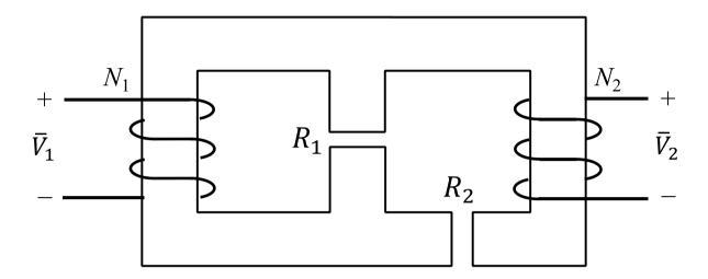
The first coil has  $N_1 = 10$  turns while the second coil has  $N_2 = 500$  turns. The transformer contains two air gaps, with reluctances  $R_1 = 50$  At/Wb and  $R_2 = 1000$  At/Wb as labeled. You may treat the permeability of the magnetic core as infinite.
