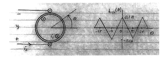
(a) Plot the open circuit voltage ( $i_s = 0$ ) as a function of  $\theta$  (label all points)
