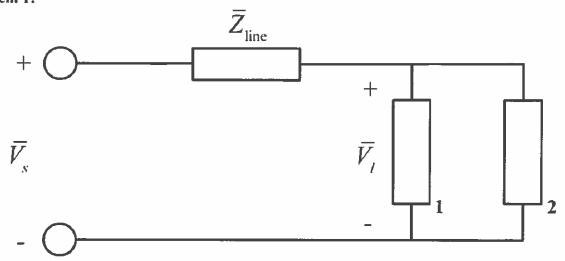
Two single-phase loads are connected in parallel to a voltage source through a feeder with impedance  $\overline{Z}_{line} = 1 + j\sqrt{3} \ \Omega$ . Load 1 consumes 1500 W of power at a power factor of 0.8 lagging. Load 2 consumes 1000 VA of power at a power factor of 0.6 lagging. The voltage at the loads is  $v_i(t) = \sqrt{2} \left(120\right) \cos\left(377t\right) V$ .
