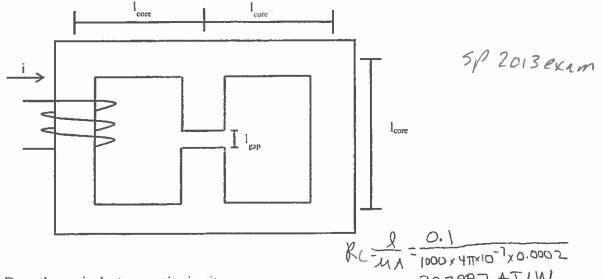
Draw the equivalent magnetic circuit.
