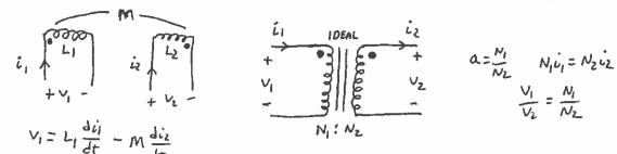
$$\alpha = \frac{N_i}{N_2} \qquad N_i \dot{v_i} = N_2 \dot{v_2}$$
