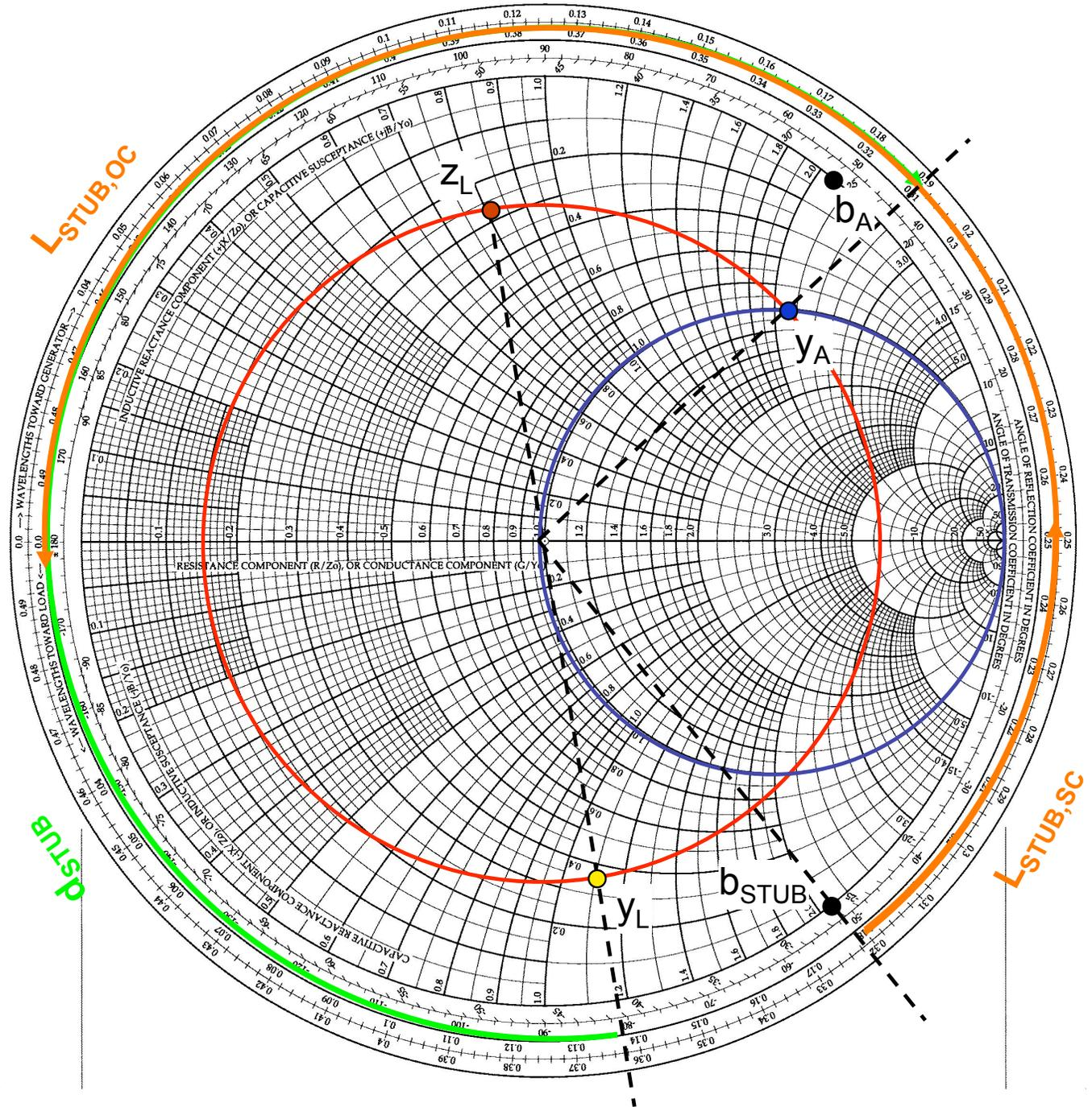
A  $50\text{-}\Omega$  T-L is terminated in an impedance of  $Z_L = 35 - j47.5$ . Find the position and length of the short-circuited stub to match it.
