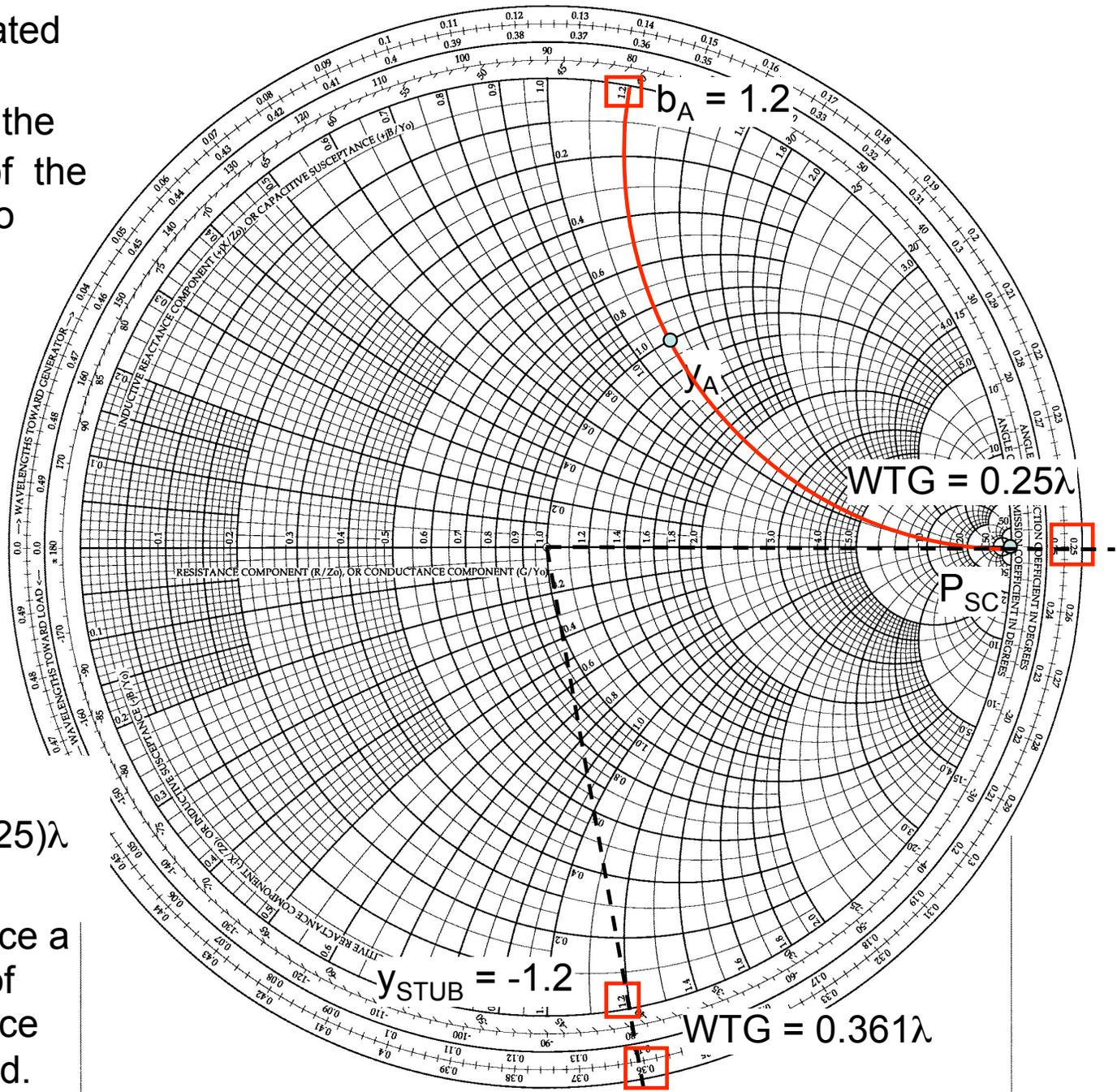
There is a second solution where the  $\Gamma$  circle and  $g=1$  circle intersect. This is also a solution to the problem, but requires a longer  $d_{\text{STUB}}$  and  $L_{\text{STUB}}$  so is less desirable, unless practical constraints require it.
