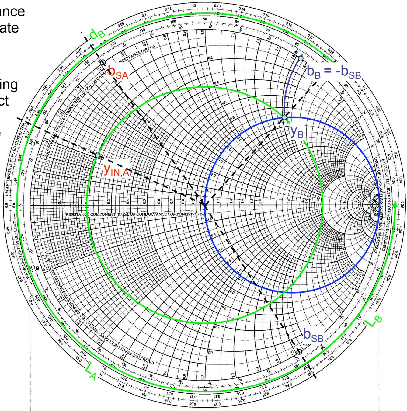
Similar to the single-stub network, there are multiple lengths for the stubs that will work.
