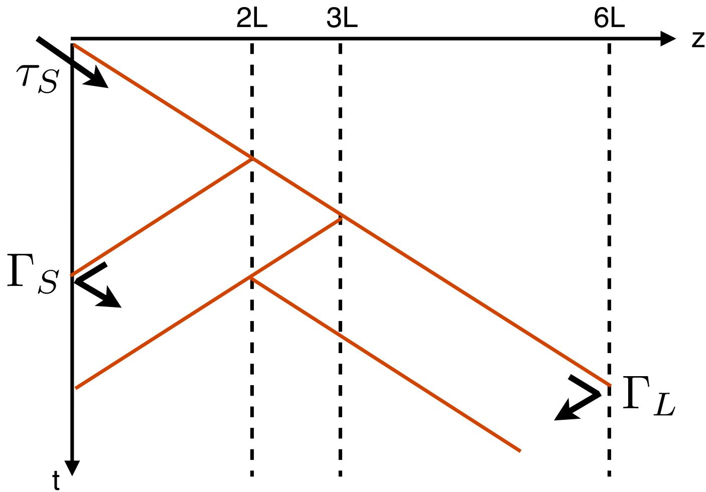
$$\Gamma_S = \frac{R_S - Z_1}{R_S + Z_1}$$
