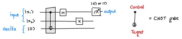
One designated qubit (say the first one) is measured in the {10>,11} basis denoted [3] and that is the output of the circuit
