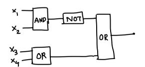
The gates only act on  $\leq 2$  bits & any function  $f: \{0,13^n \rightarrow \{0,13\}$ can be computed by some circuit on n bits
