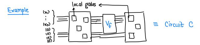
Note that  $V_f$  "computes" the true value of the function so the quantum circuit can use these true values in intermediate superpositions
