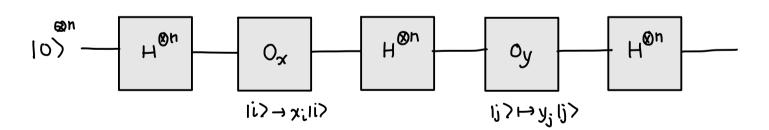
The final state of this circuit (before measurement) in the computational basis 10>, 11>, --- 1N> looks like
