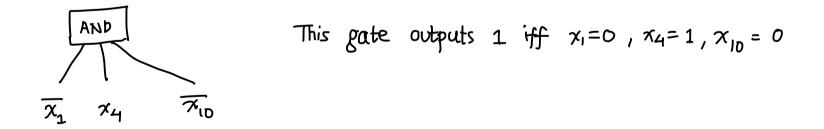
We add such AND gates for each accepting path and then add a single OR gate in the top layer connected to all the AND gates
