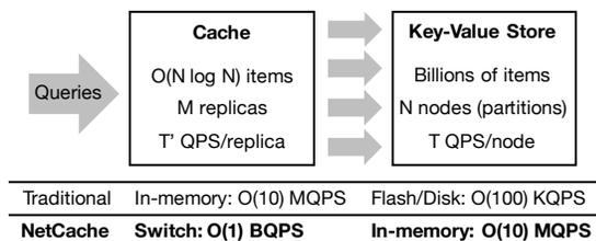
**Figure 1: Motivation. To provide effective load balancing, a cache node only needs to cache  $O(N \log N)$  items, but needs to be orders of magnitude faster than a storage node ( $T' \gg T$ ). NetCache caches data in the network when key-value stores move to the memory.**
