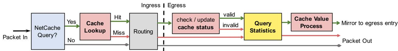
Figure 8: Logical view of NetCache switch data plane.
