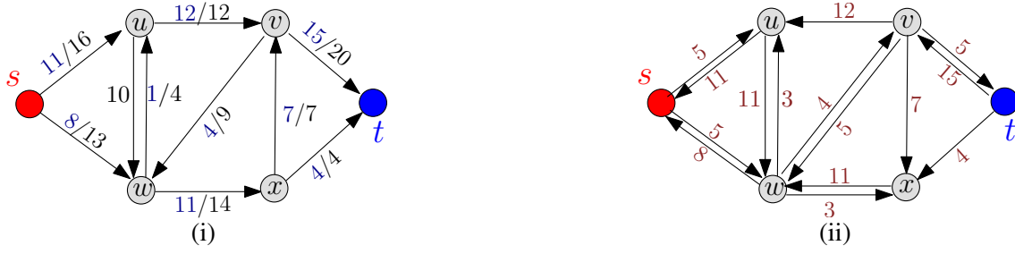
Figure 16.2: (i) A flow network, and (ii) the resulting residual network. Note, that f(u, w) = -f(w, u) = -1 and as such c_f(u, w) = 10 - (-1) = 11 .
