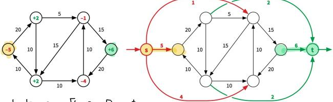
b(v) - balance = Flow in - Flow out
