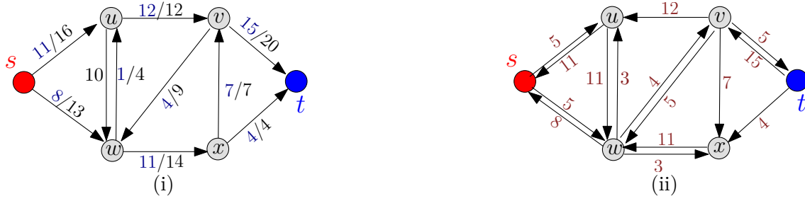
Figure 17.2: (i) A flow network, and (ii) the resulting residual network. Note, that f(u, w) = -f(w, u) = -1 and as such c_f(u, w) = 10 - (-1) = 11 .
