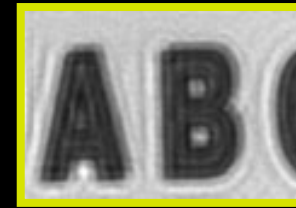
Ringing with the traditional Richardson-Lucy deconvolution algorithm
