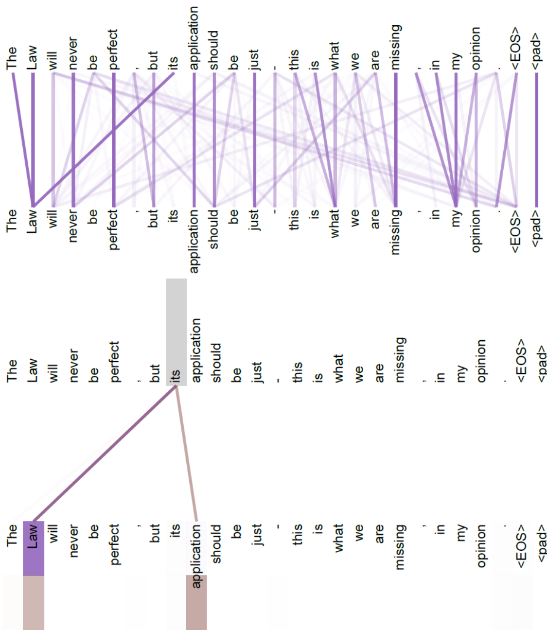
Figure 4: Two attention heads, also in layer 5 of 6, apparently involved in anaphora resolution. Top: Full attentions for head 5. Bottom: Isolated attentions from just the word 'its' for attention heads 5 and 6. Note that the attentions are very sharp for this word.
