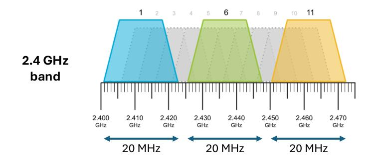
APs and devices on the 2.4 GHz band should operate on these channels to reduce interference
