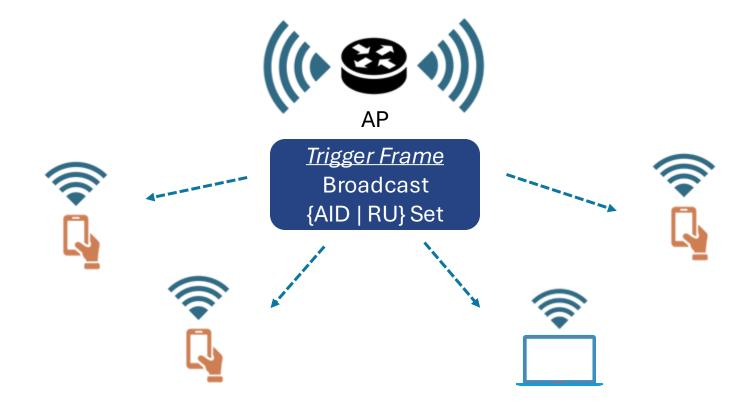
RUs are allocated by the AP, determined by traffic demand Trigger Frames define the RUs that devices can use
