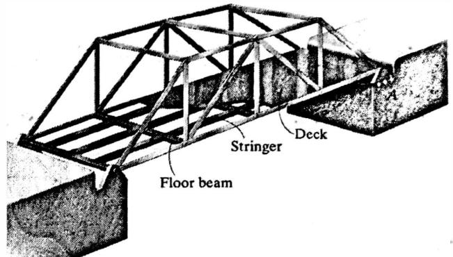
To analyze the design of a truss, we will work through a **free-body diagram** including reaction forces, followed by **equations for equilibrium**, and determine **reaction forces at the supports** and **internal forces** on the supporting side truss members. For everything ahead, we will simplify the problem by considering it in 2D.
