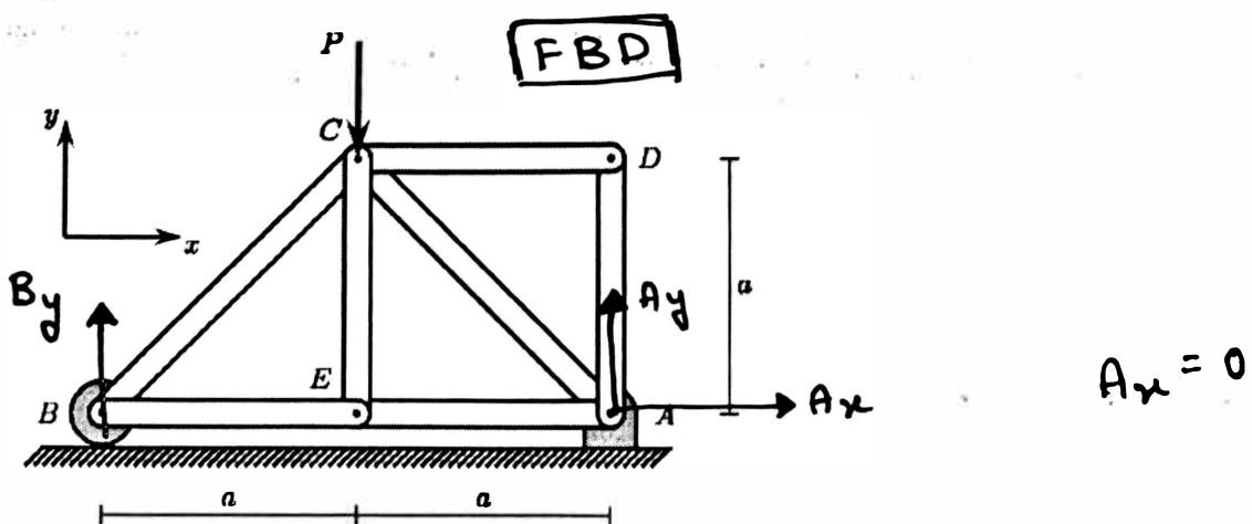
2) Use the FBD from Question 1 to find the support reaction forces at  $A$  and  $B$  in terms of the load  $P$  and distance  $a$ .
