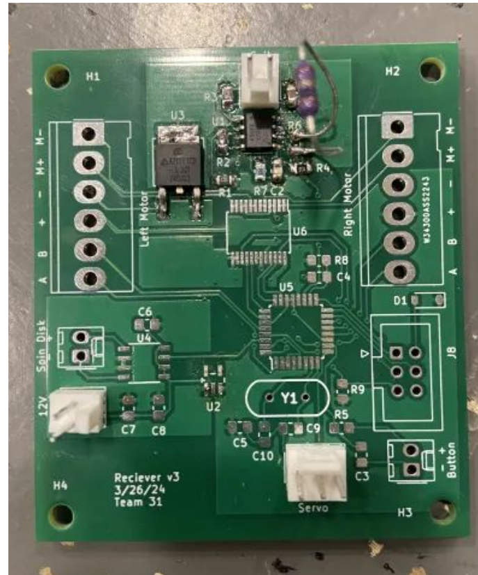
Receiver Board used in the sensing demo
