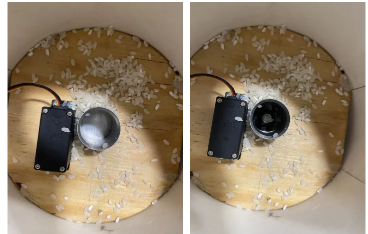
Closed and open state of the dispenser flap
