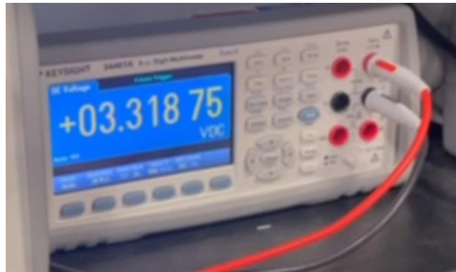
Figure 12: 3.3 volts from the linear voltage regulator.
