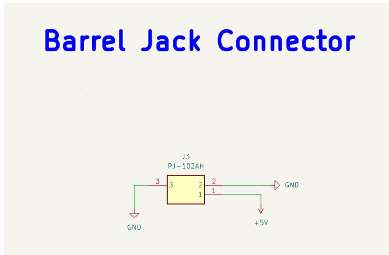
Figure 2: Barrel Jack Connector Schematic
