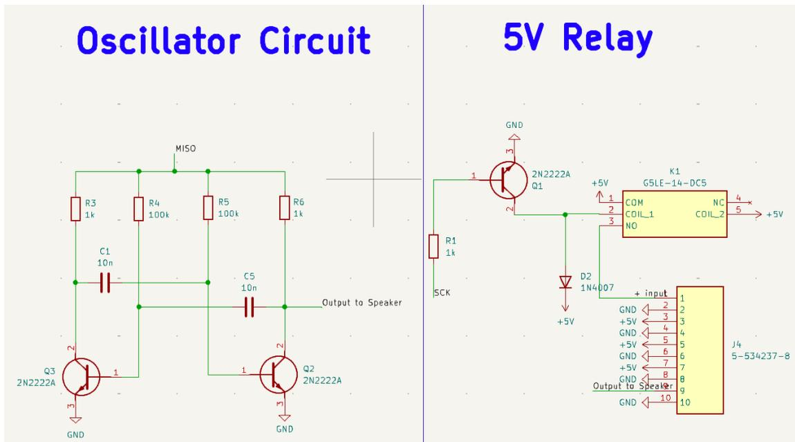
Figure 5: Oscillator Circuit and 5-Volt Relay Schematic
