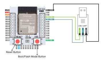
Figure 8: Connecting esp32 with the USB/UART bridge
