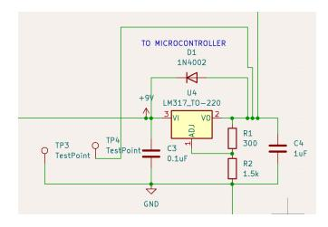
Figure 3: Linear Regulator LM317 Schematic
