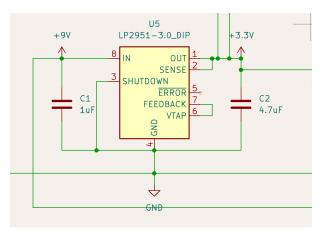
Figure 2: Linear Regulator LP2951 Schematic
