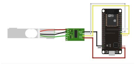
Figure 5: Load cell, HX711 and ESP32 Configuration
