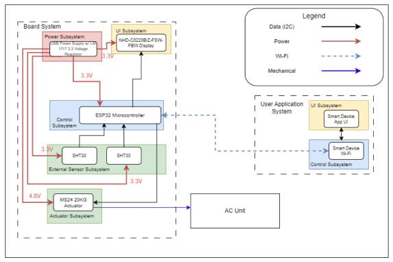
Figure 4 - Block Diagram of Smart AC Device
