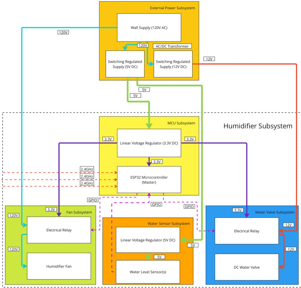
Figure 4 – Humidifier Subsystem Block Diagram (Close-up) [16]
