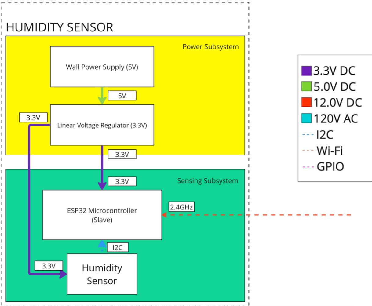
Figure 5 – Humidity Sensor Subsystem Block Diagram (Close-up) [15]
