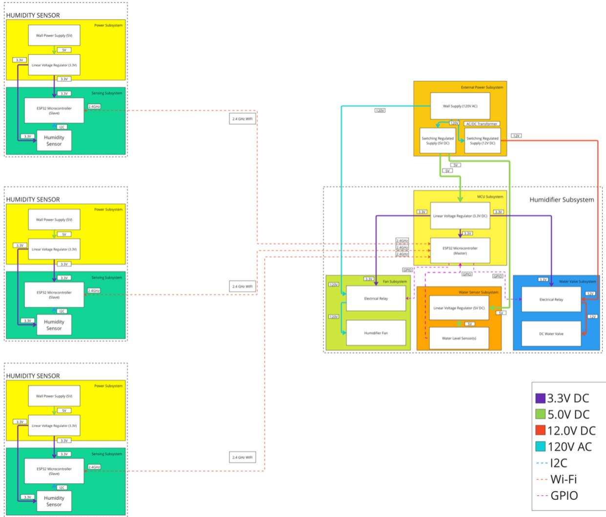
Figure 3 – Overall Block Diagram [28]
