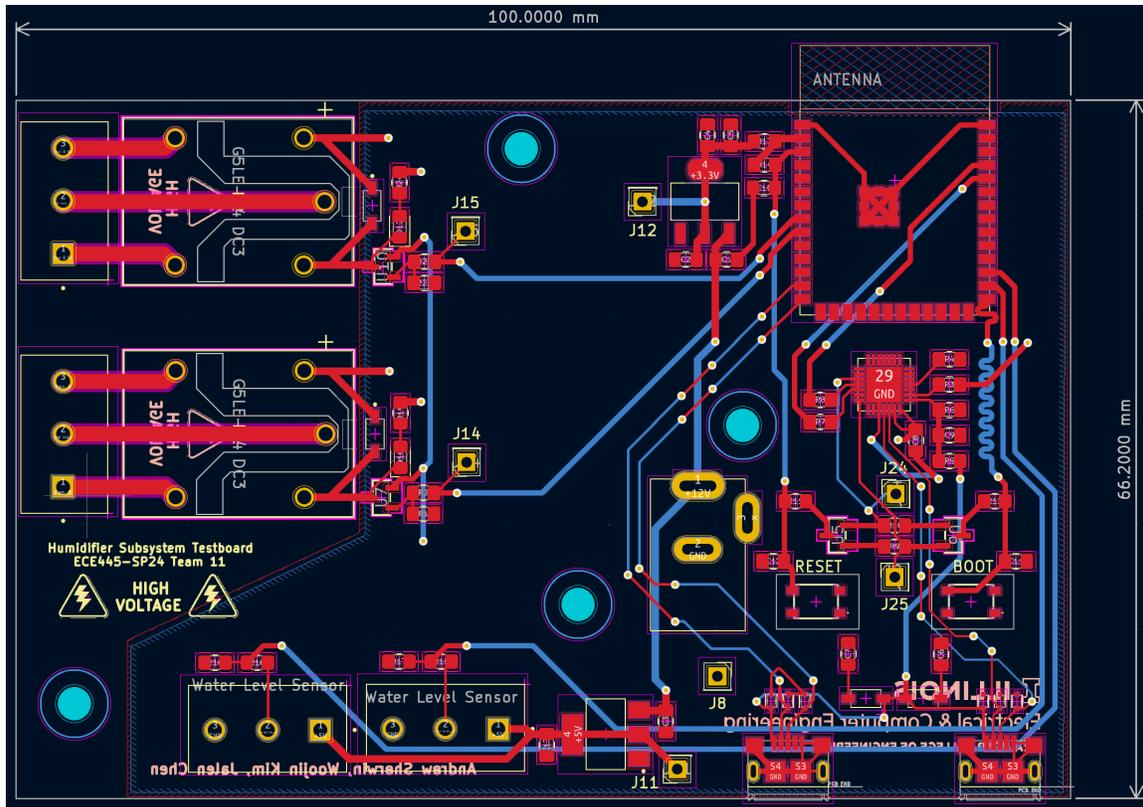
Figure 6 – Humidifier Subsystem PCB [29]
