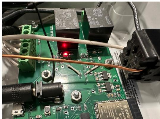
LED light when valve is on
