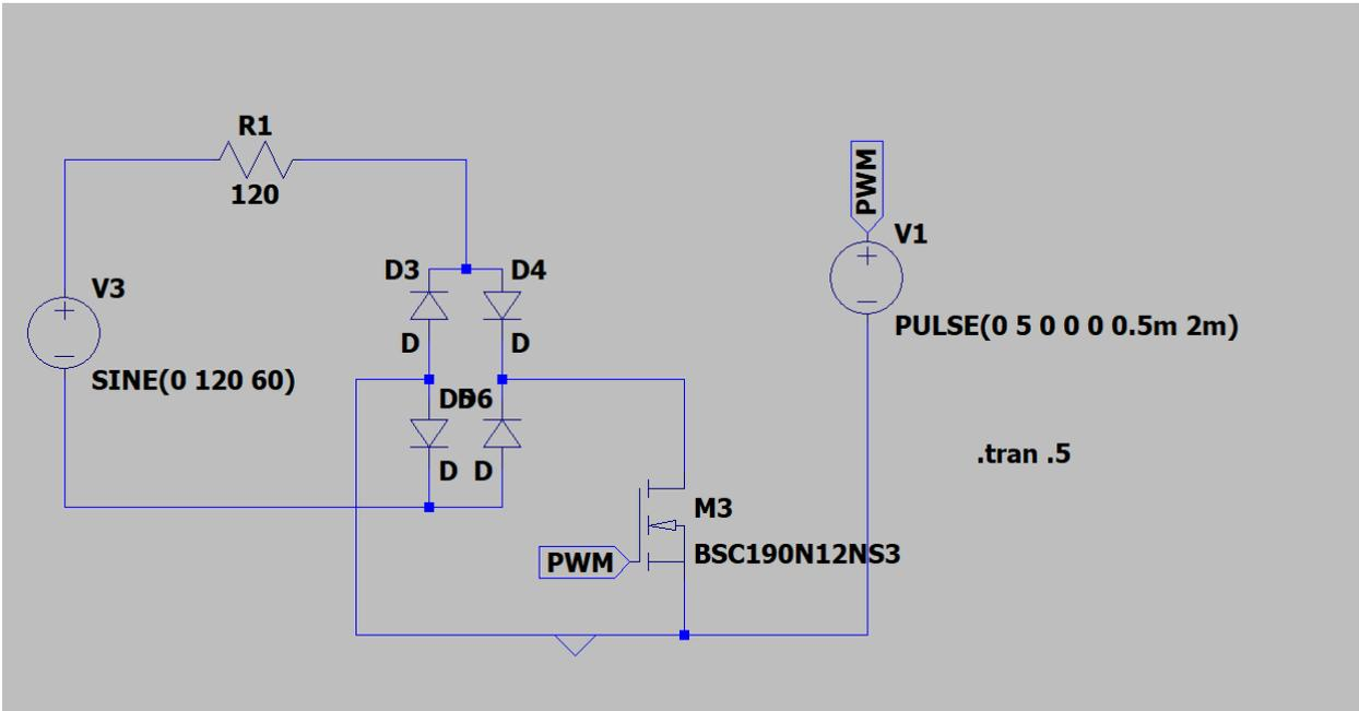
Fig. 4a. AC Pulse Width Modulation circuit using MOSFET.
