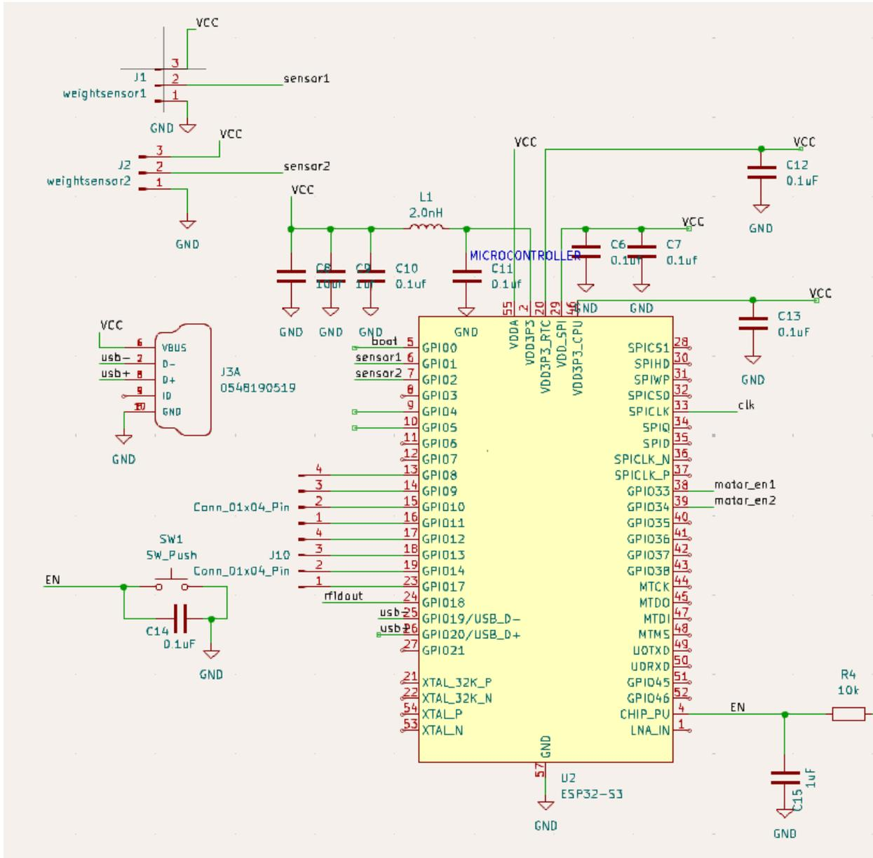
Fig 2: Control System with USB outputs
