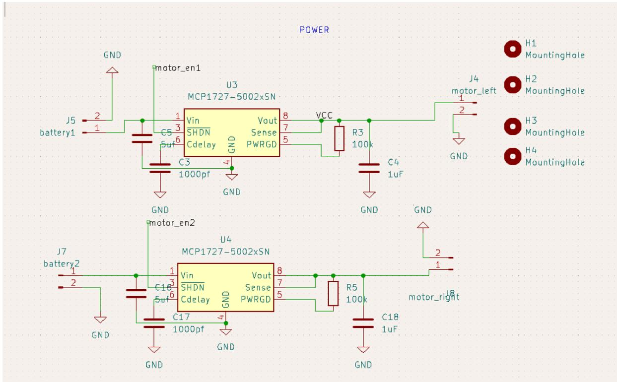
Fig 1: Power system and linear regulators
