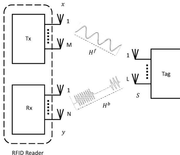
We can make sure that either the frequencies from the tags are different so much that the reader will not mix them or we can make the reader accurate in detecting the different frequencies.
