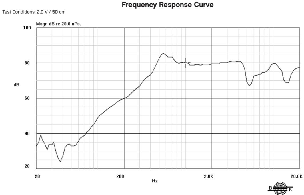
Figure 4: Speaker's response (dB) to different frequencies (Hz)
