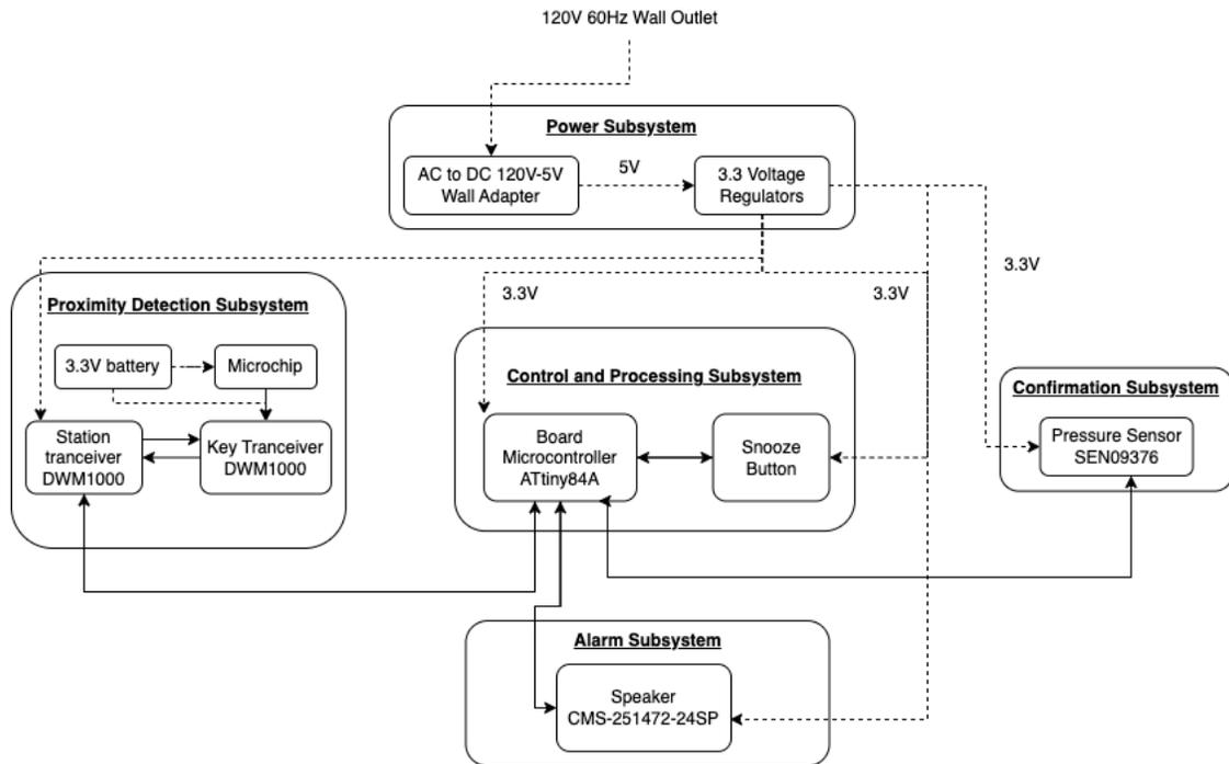
Figure 3: Block diagram outlining subsystem connection
