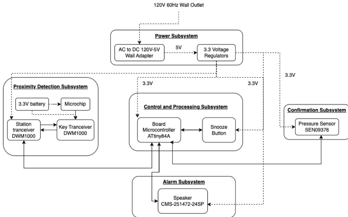
Figure 3: Block diagram outlining subsystem connection
