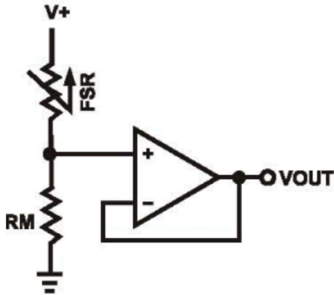
Figure 7: Force-Sensing Resistor Schematic
