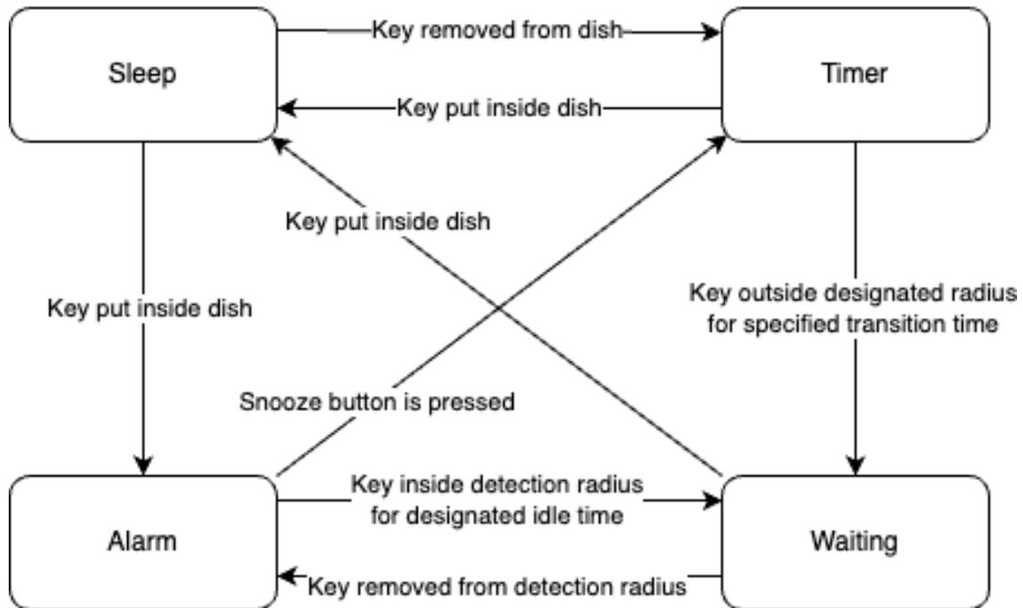
Figure 5: State diagram of dish
