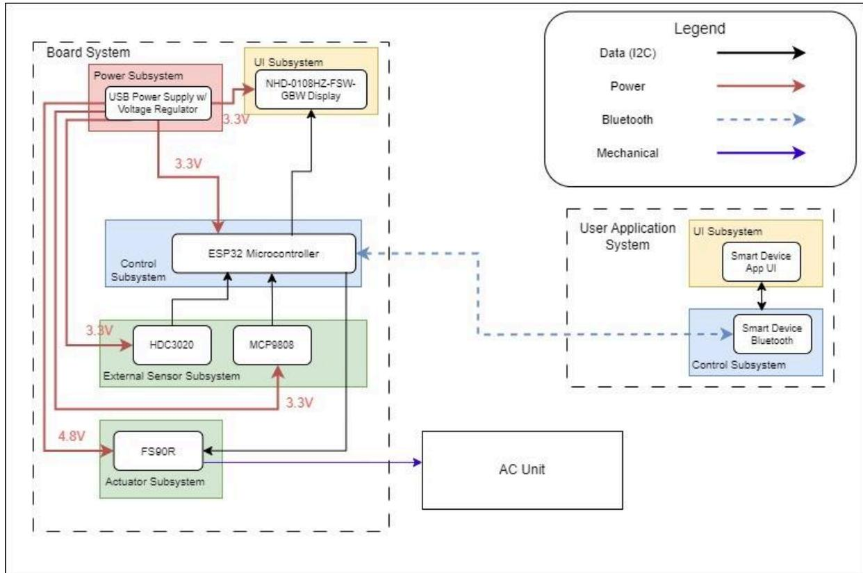
Figure 3 - Block Diagram of Smart AC Device
